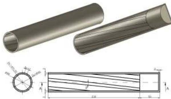
Figure 2: Cross-section of a rifled weapon barrel
