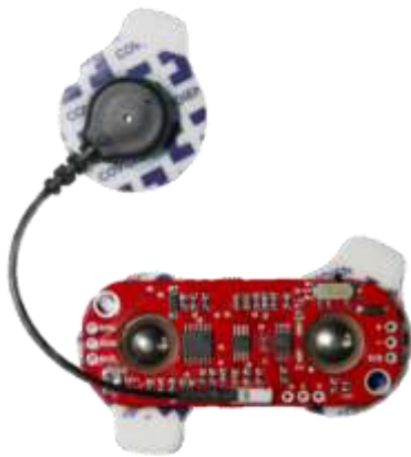
Figure 3: MyoWare Muscle Sensor used for muscle voltage signal acquisition [25]
