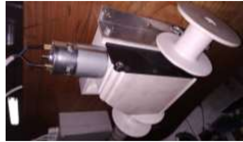
Figure 9: Motor with gear assembly mounted under the tabletop of the standing frame
