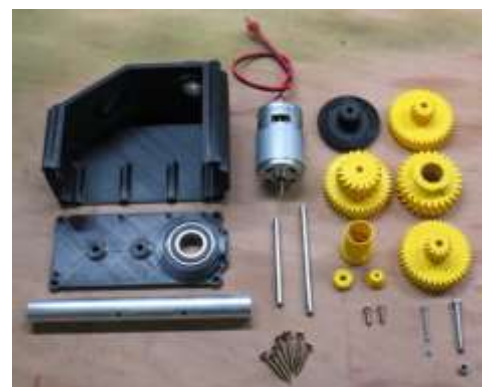
Figure 6: Components of the verticalizing (lifting) mechanism [20]
