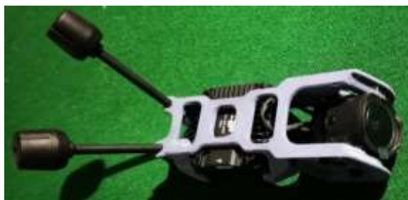
Figure 8: Preliminary prototype of the imaging system with Dji O4 Air Unit Pro module mounted in an open housing
