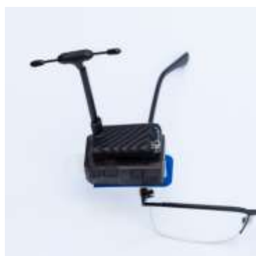
Figure 4: Head-tracking unit mounted on eyeglass frame
