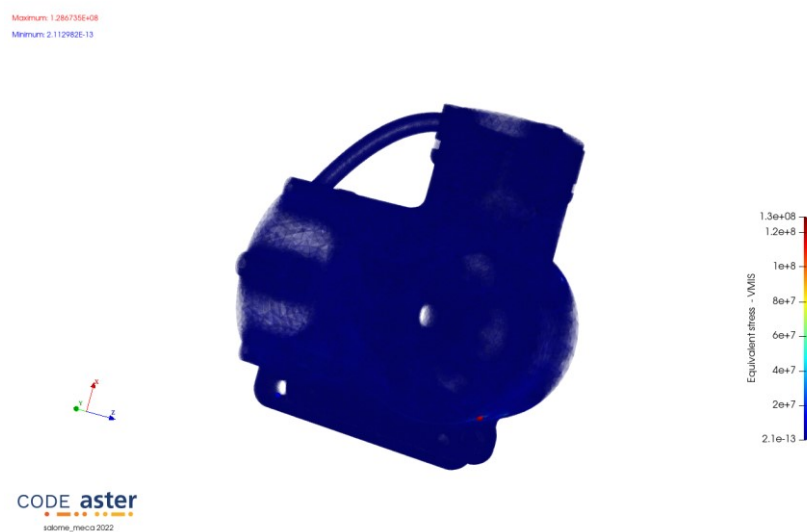
Figure 8: Representation of maximum and minimum stresses on the motor body (according to the Von Mises criterion)
