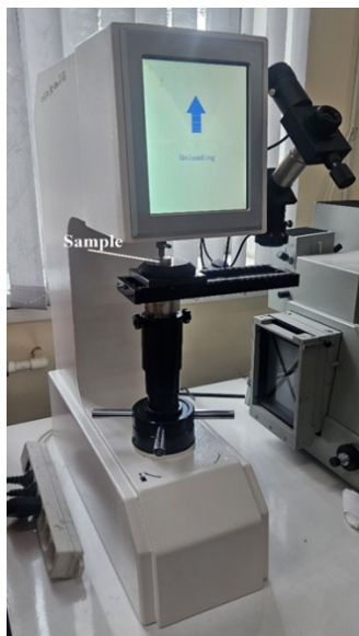
Figure 5: THBRV-187.5DX hardness testing device
