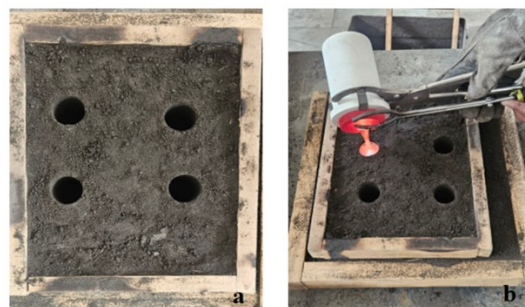
Figure 3: a — sand-clay mold; b — sample casting process
