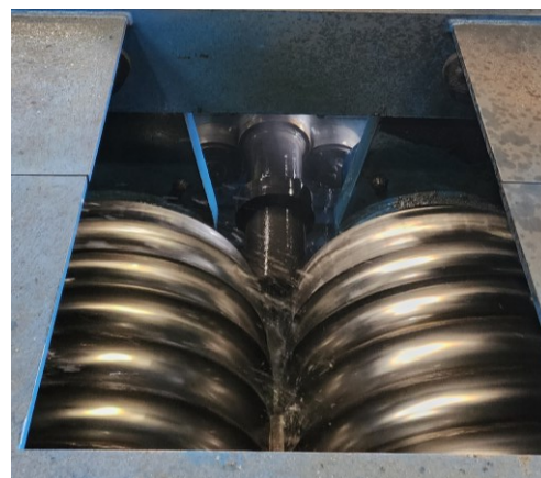
Figure 1: General view of ball rolling mill rolls
