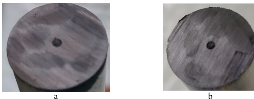
Figure 9: Investigation of surface burns using SL3 lubricant: (a) – initial sample with burns; (b) – surface after treatment with etching solution.
