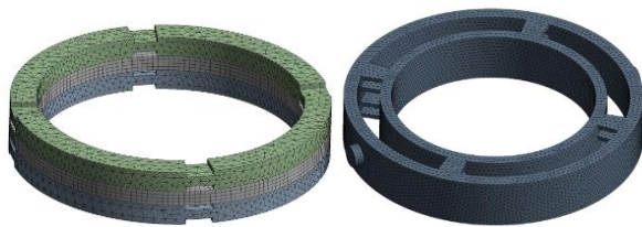
(a) Mesh of the Friction Pair (b) Mesh of the Lubricating Oil Figure 3: Meshes of the Friction Pair and Lubricating Oil
