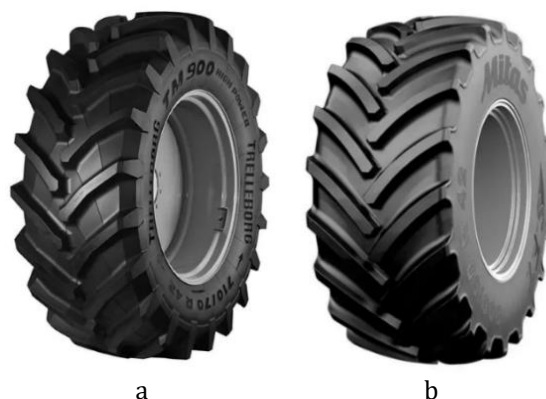
Figure 3: Tested rear tires Trelleborg 710/75 R42(a) and Mitas 710/70 R42(b)
