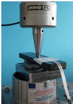
Figure 2: FlexiForce A201 force sensor installed on the Instron 8872 fatigue testing system.
