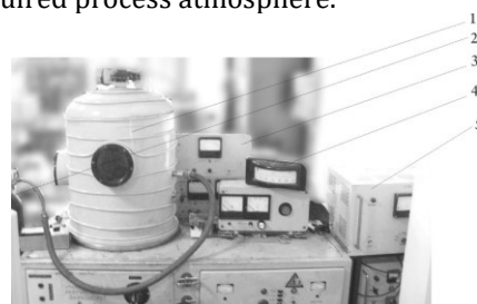
Figure 2: Experimental setup: 1 – vacuum chamber; 2 – gas supply equipment; 3 – VT-2A-P vacuum gauge; 4 – temperature control device; 5 – glow discharge power source
