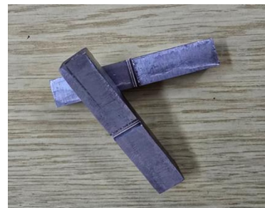
Figure 5: Charpy impact test specimens prepared for impact toughness evaluation
