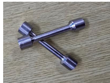
Figure 4: Dog-bone-shaped tensile test specimens prepared for tensile strength testing.
