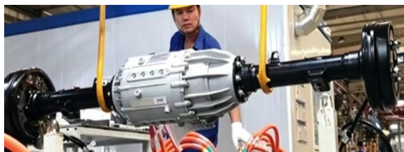
(a) Physical prototype of the drive axle
