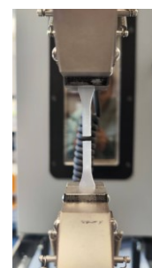
Figure 3: Fracture of the sample after tensile test
