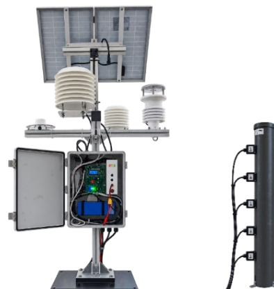
Figure 2: Experimental IoT soil-monitoring station developed by the authors.
