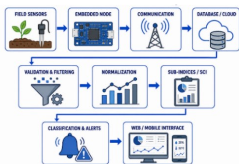
Figure 1: General architecture of the proposed IoT-based soil condition assessment system
