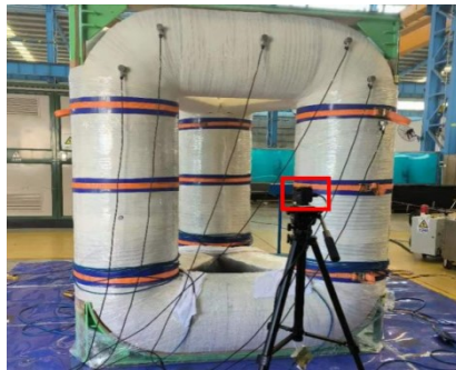
(a) Acoustic measurement-point arrangement
