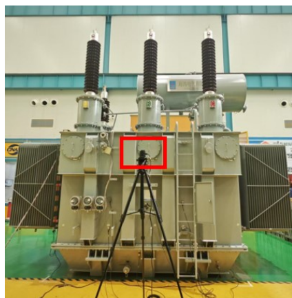
(a) Acoustic measurement-point arrangement
