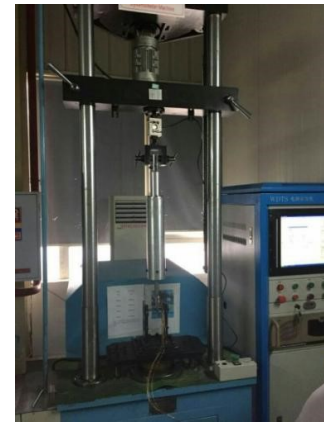
Figure 17: Bench test of the actuator
