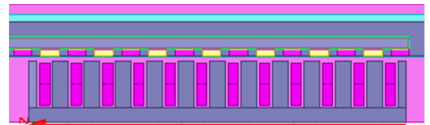
Figure 4: Finite element model of the actuator
